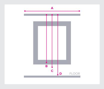
**Step 1:** Measure the full width of the curtain track from end to end using a metal tape measure (A).
