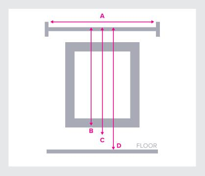
**Step 1:** Measure the width between the end caps of the curtain pole (A).
